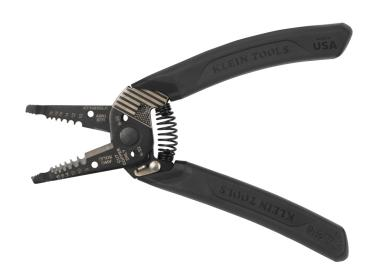
The Klein-Kurve Limited-Edition Blackout Wire Stripper / Cutter combines precision and versatility with six stripping holes for 8-18 AWG Solid and 10-20 AWG Stranded wire, dual looping holes for easy connections, and screw shearing for 6-32 and 8-32 bolts. Longer blackout handles and a narrow head design provide comfort and allow access to tight spaces, while a coil spring and convenient lock ensure smooth operation and easy storage.
